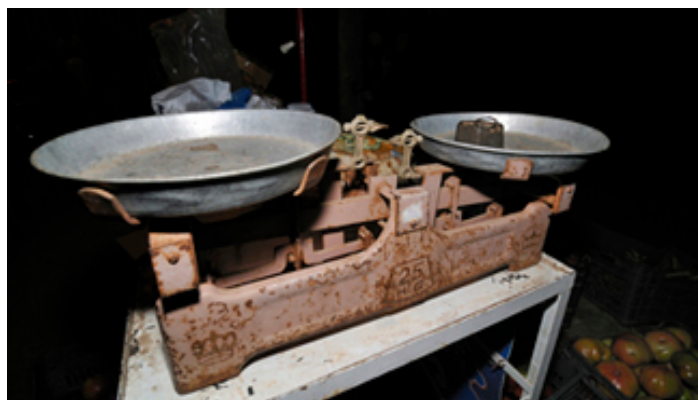
Figure 1.22 A double-pan mechanical balance is used to compare different masses. Usually an object with unknown mass is placed in one pan and objects of known mass are placed in the other pan. When the bar that connects the two pans is horizontal, then the masses in both
